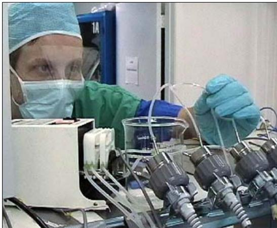
A technician checks lines connected to electronic devices that measure cryoprotectant concentration (refractometers).
