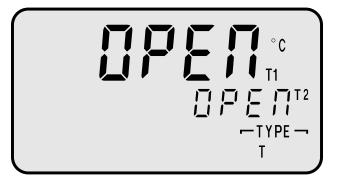
This display shows that both ports are open, and no thermocouple probes have been connected. If you see this, check the connections.
