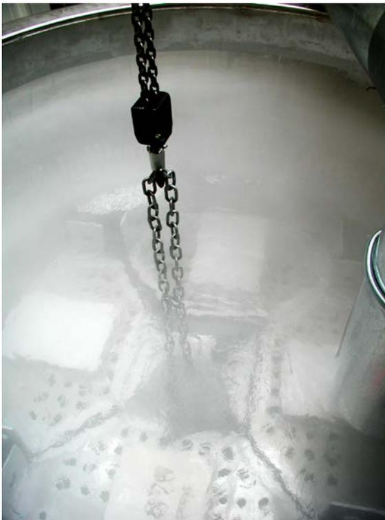
*Figure 20-20. The neuro column after being lowered back into a bigfoot dewar.*
