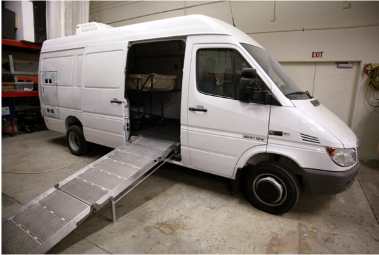
Figure 17-15. Custom-built aluminum ramp extended from the side door of the Sprinter van acquired by Suspended Animation.
