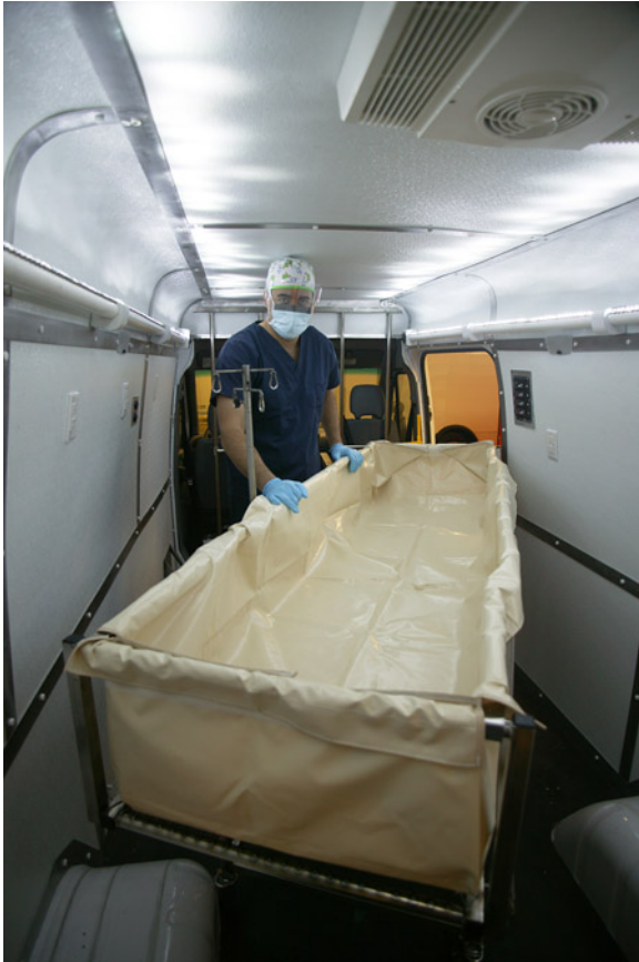
Figure 17-16. The interior of the Sprinter van after its initial conversion at Suspended Animation. The walls have been panelled with washable plastic, and LED lighting has been installed. An aftermarket air conditioner is visible in the roof.
