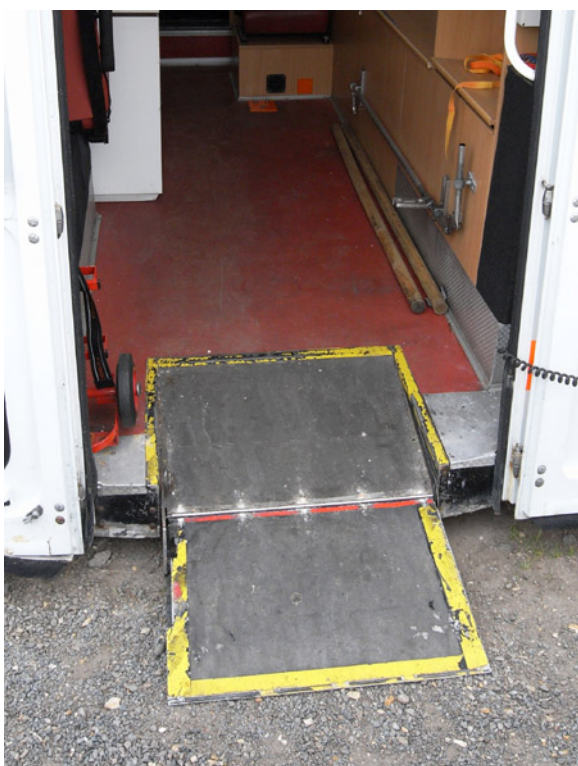
Figure 17-20. The ramp folded down in Alan Sinclair’s ambulance.
