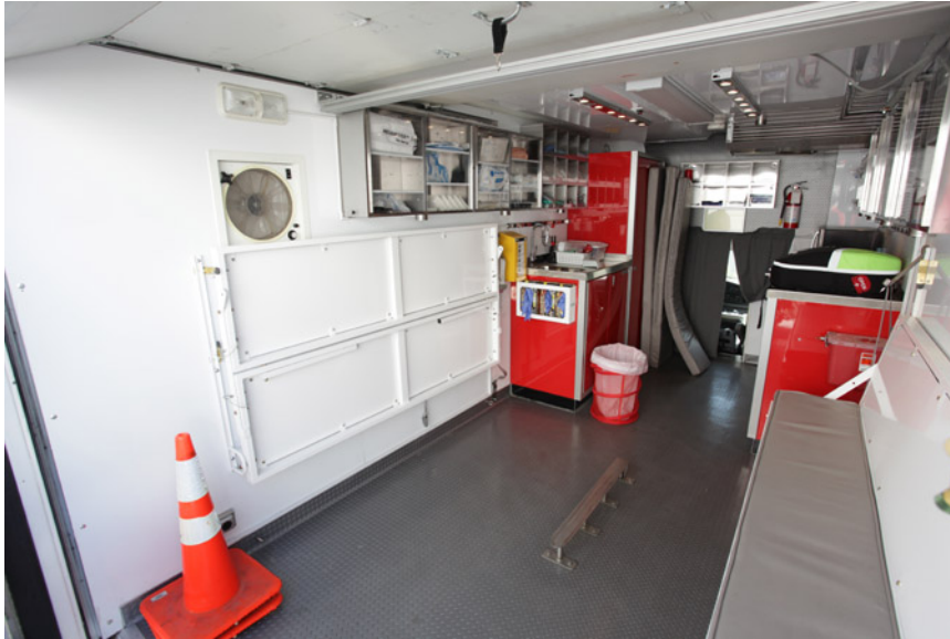
Figure 17-10. Interior of the Alcor patient transport vehicle with one seat folded up to allow the ice bath to be loaded.
