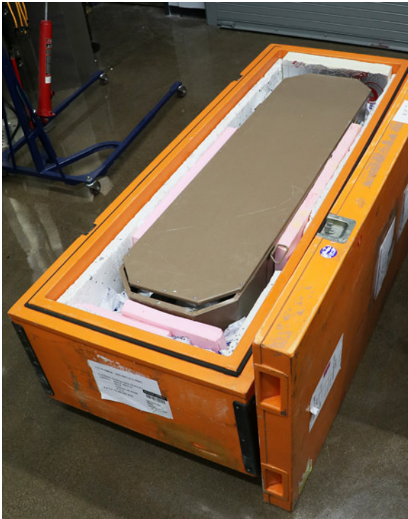
Figure 17-6. A whole-body dry-ice shipping container designed and built by Alan Sinclair in the UK. A Ziegler box is visible inside it. This particular photograph shows gaps in the foam insulation surrounding the Ziegler case. It should be noted that this is highly undesirable for insulating efficiency because even small air gaps between insulating panels will support heat transport by passive convection. This can be ameliorated by interleaving small gaps between two or more panel layers so that there are no gaps directly connecting the shipping container interior and exterior.
