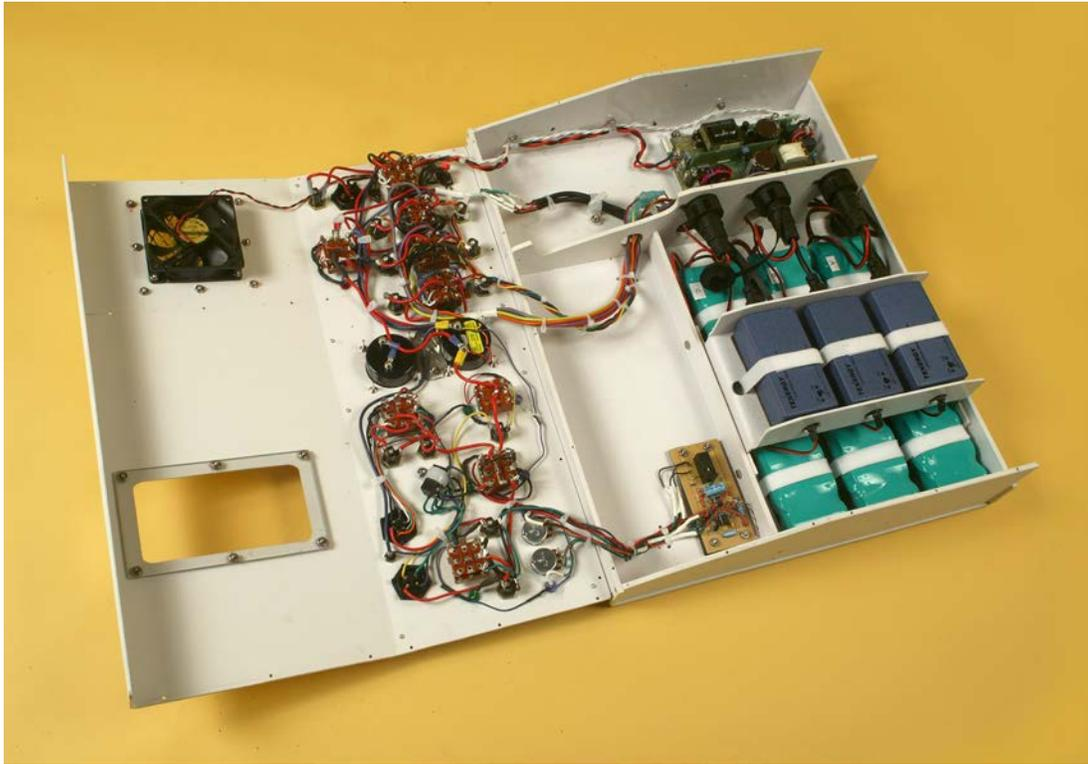
*Figure 12-6. The control panel for LV2, opened to reveal three battery packs and chargers, an AC-DC converter in a separate compartment, and very simple control electronics on a 2x4 inch circuit board.*
