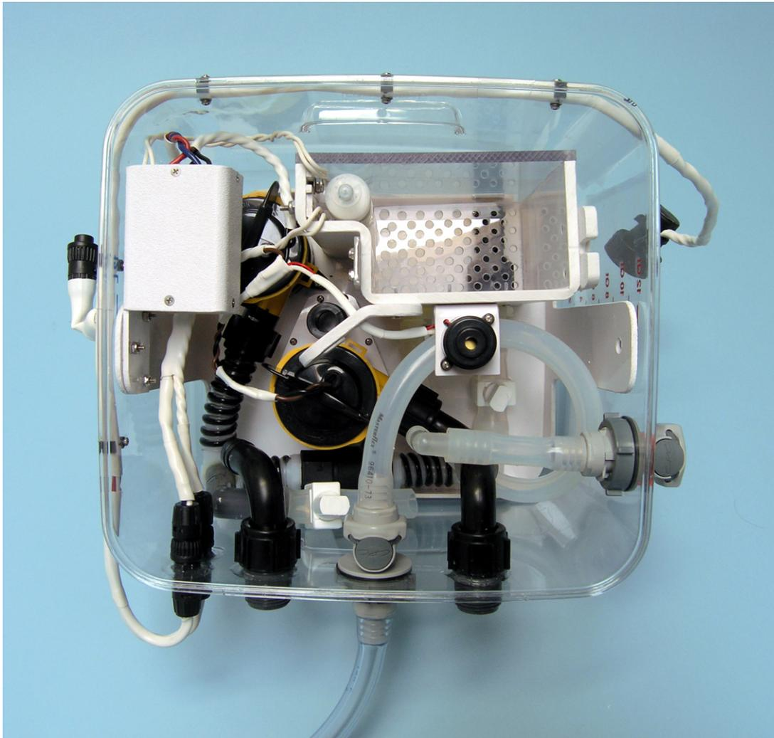
*Figure 12-11. Overview of the perfluorocarbon reservoir in LV3. The sub-reservoir at top right was enlarged relative to the infusion reservoir in LV2, to provide sufficient capacity for cryonics cases, although the system was never used for this purpose.*
