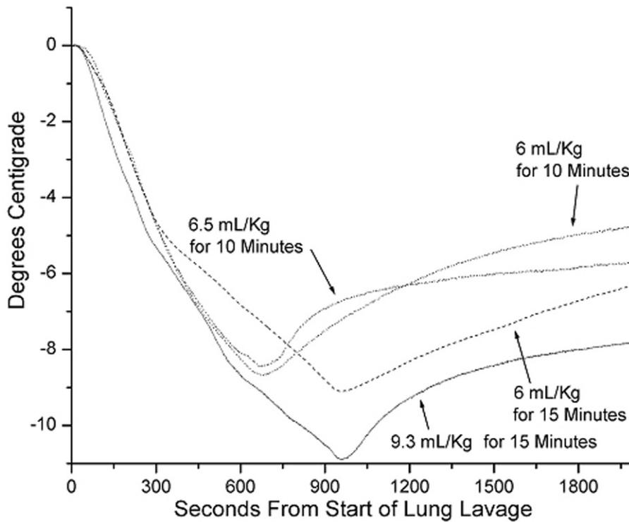
*Figure 12-1. Cooling curves from experiments with liquid ventilation devices. These curves were submitted with an international patent application in 2008. A peak cooling rate of greater than 1 degree Celsius was achieved repeatedly, and even at the lower temperature range of 9 to 11 degrees below normal body temperature, the lowest of the curves shows that a rate of approximately 2 degrees in 5 minutes was recorded (0.4 degrees per minute). Temperatures were measured tympanically.[3]*
