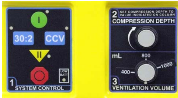
Figure 9-8. Control panel for the Life-Stat.
