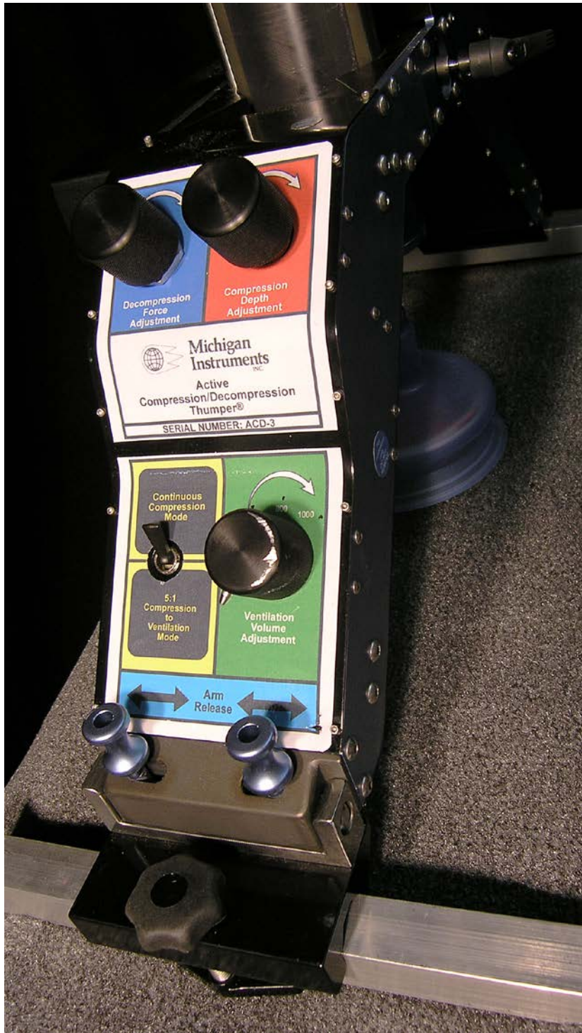
Figure 9-14. Controls on the Suspended Animation ACDC Thumper.
