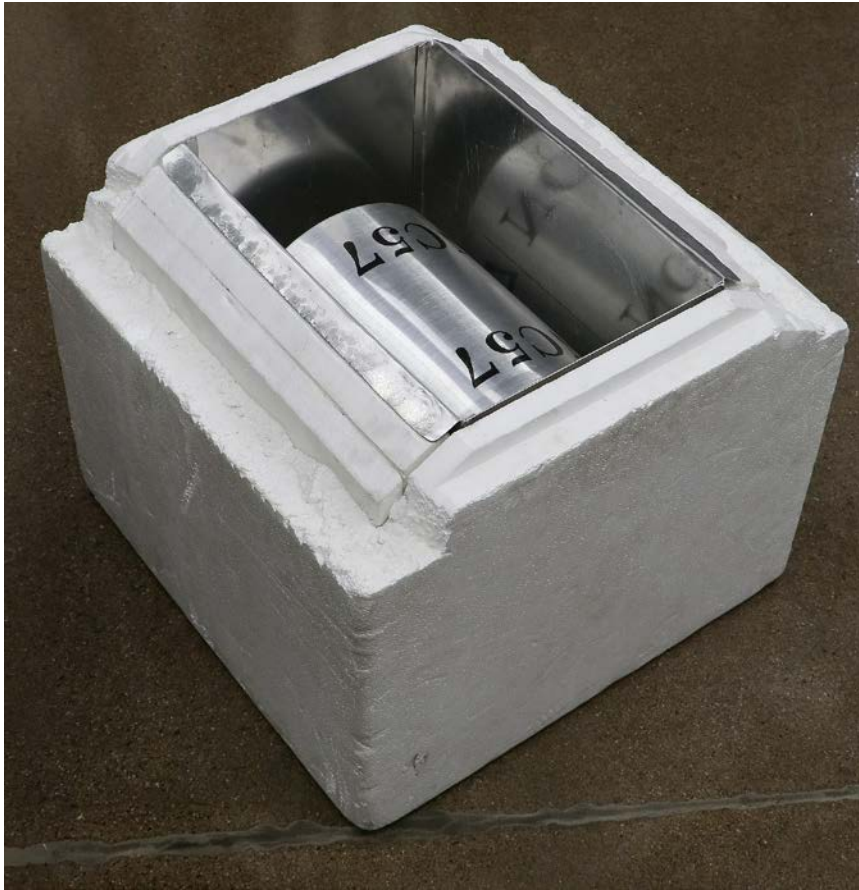
Figure 20-21. A neurocanister is immersed in liquid nitrogen in this styrofoam carrier when it is passed through a CT scanner.
