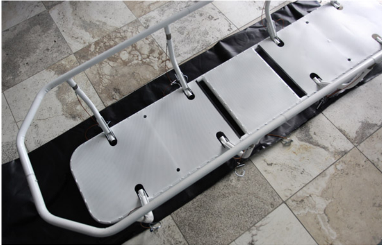
Figure 11-29. The frame of Graber's ice bath, attached to its baseplate.
