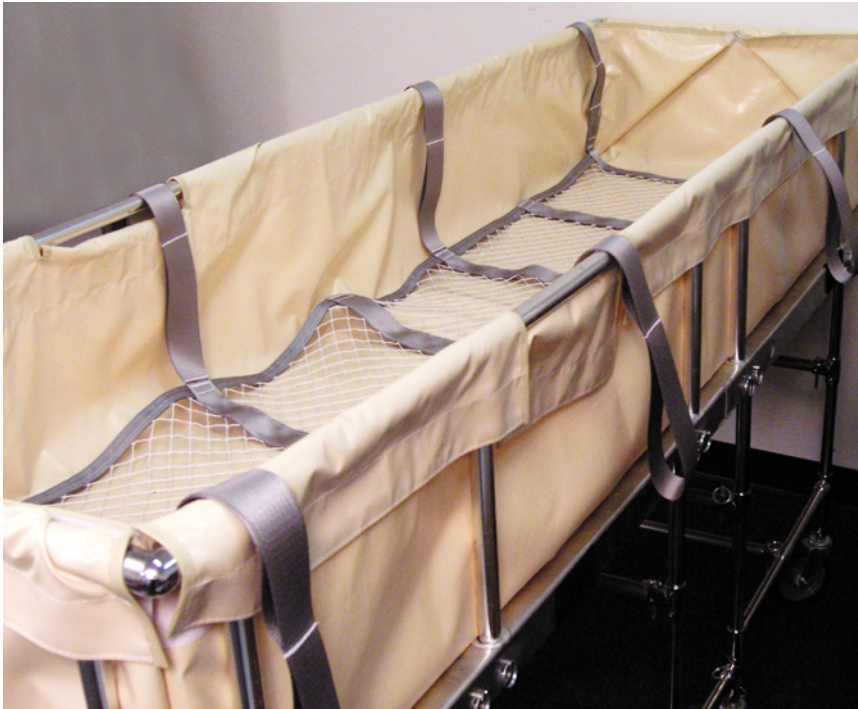
Figure 11-3. A lifting sling fabricated from nylon webbing and netting is shown in an ice bath at Suspended Animation, Inc.
