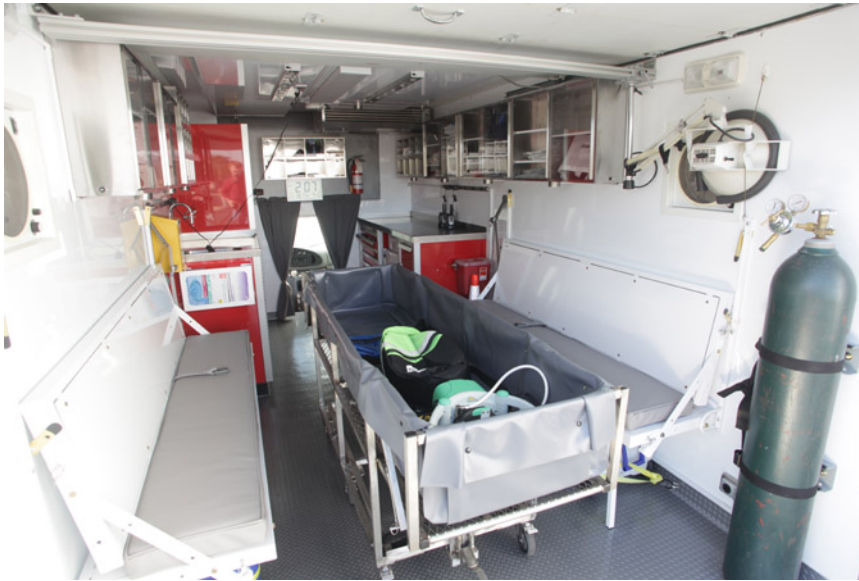
Figure 17-12. The ice bath loaded into the Alcor vehicle, and the seats folded down.
