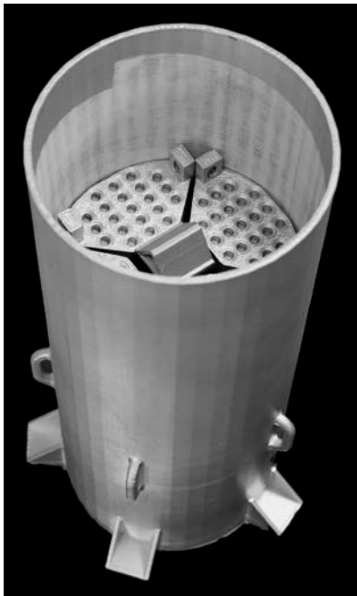
Figure 20-12. This 3D print by Steve Graber at Alcor shows how the pods and neuro column fit into a bigfoot.
