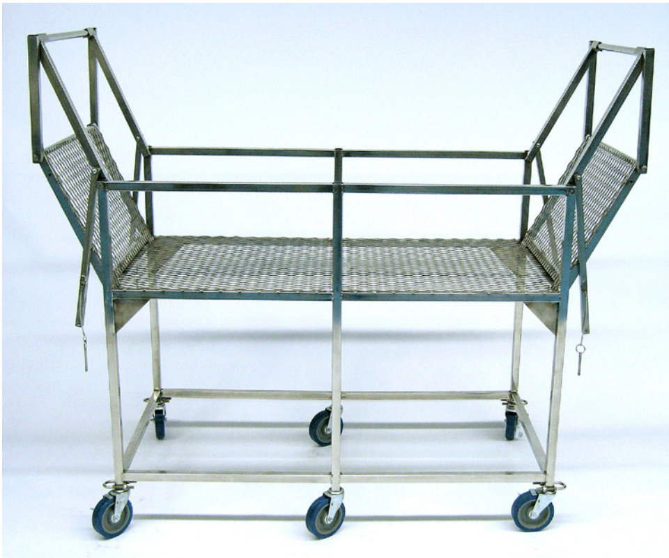
Figure 11-22. Ends of the noncollapsible ice bath in Figure 11-22 could be turned upward to reduce the length when necessary.
