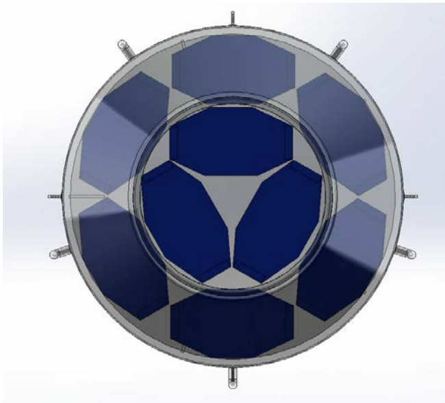
Figure 20-16. The proposed packing arrangement for patient pods in the SuperD dewar.
