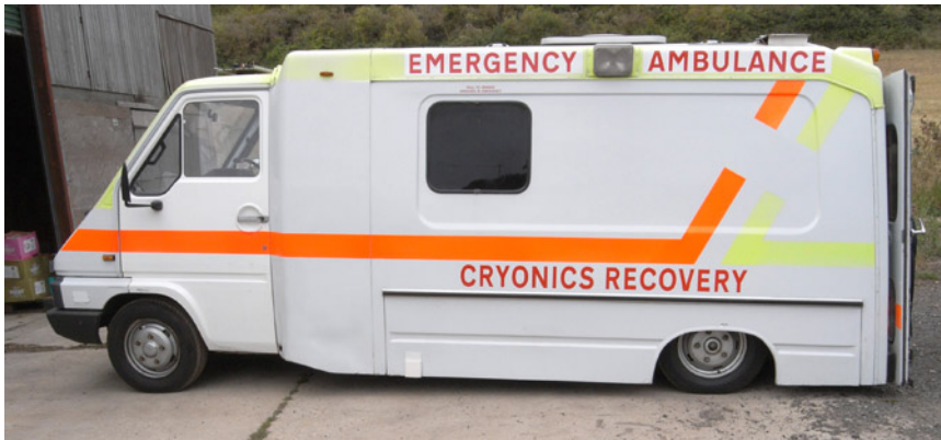
Figure 17-18. The ambulance converted by Alan Sinclair in the UK, shown with its rear suspension in the lowered position.
