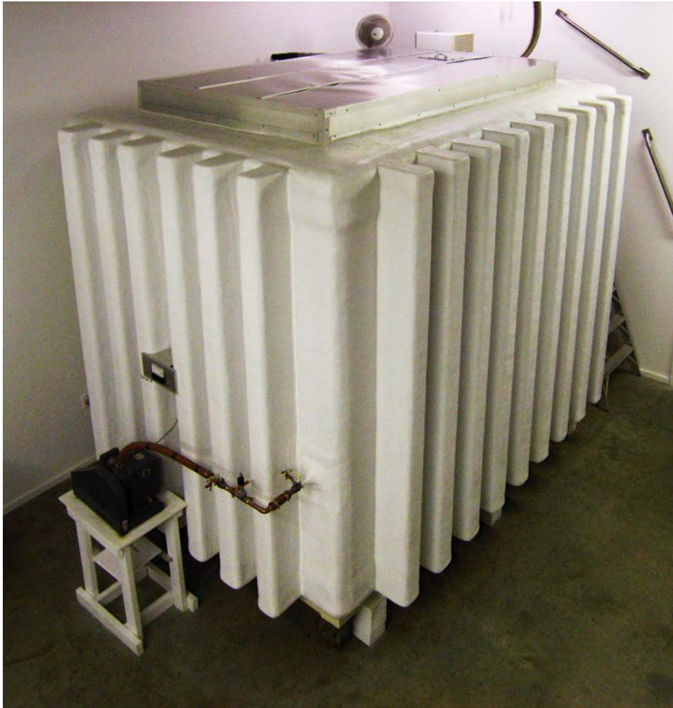
Figure 20-29. The largest of the cryostats at the Cryonics Institute. A vacuum pump stands on a small table at bottom-left.
