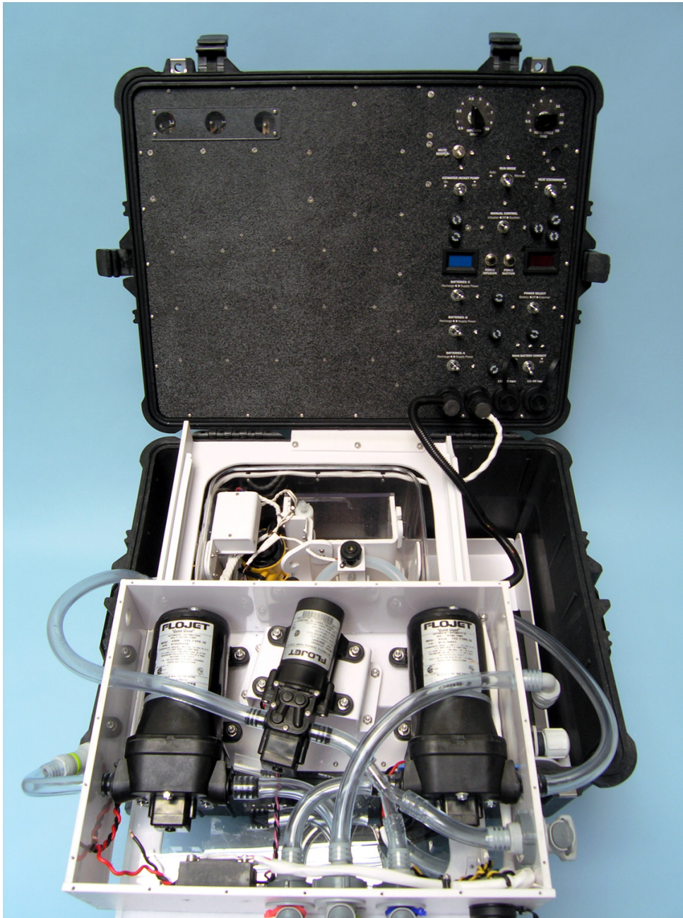
Figure 12-9. The pump box for LV3 was located on a platform that could slide out to allow access to the perfluorocarbon reservoir below. The whole assembly was designed to sit above the patient's legs on the rails of a portable ice bath, but its elevation greatly reduced the efficiency of suction from the lungs..
