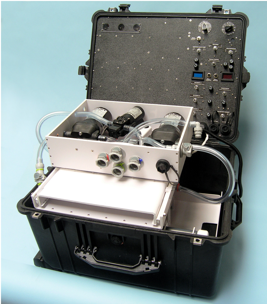
Figure 12-8. In LV3, batteries and chargers were mounted inside the lid of the primary Pelican container, alongside switches and control electronics. A more powerful infusion pump and a more powerful suction pump than in LV2 were mounted in a separate box, together with a small pump that cooled an icewater jacket on the delivery tube (the tube is not shown here).
