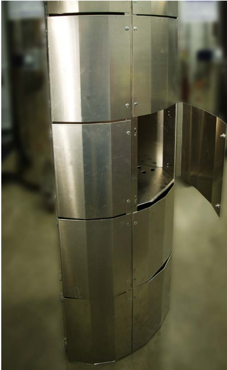
Figure 20-10. A whole-body pod can be reconfigured to hold 10 neuropatients, each in a separate compartment.
