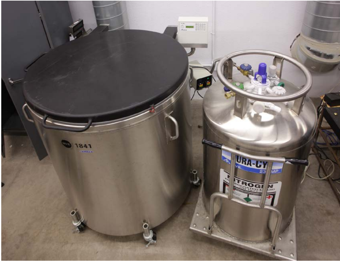
Figure 20-26. The dewar adapted for intermediate temperature storage stands beside a small dewar of liquid nitrogen in Alcor's patient care bay.
