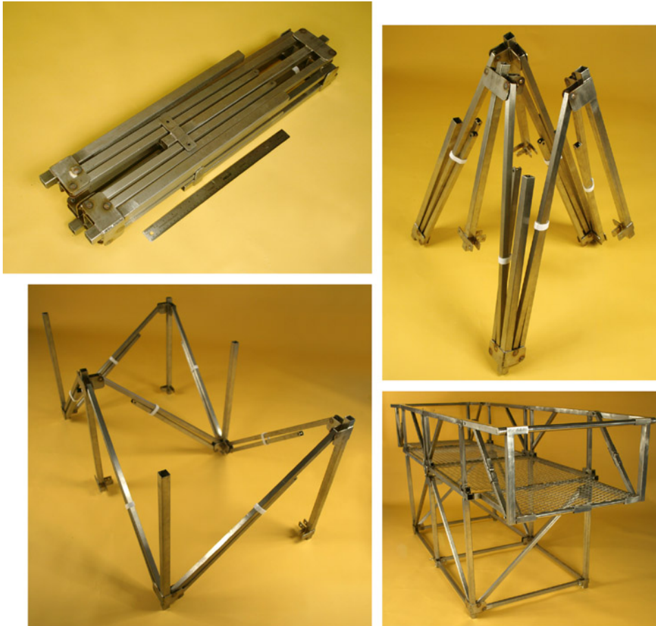
Figure 11-20. A foldable set of legs for the ice bath shown in Figure 11-19.
