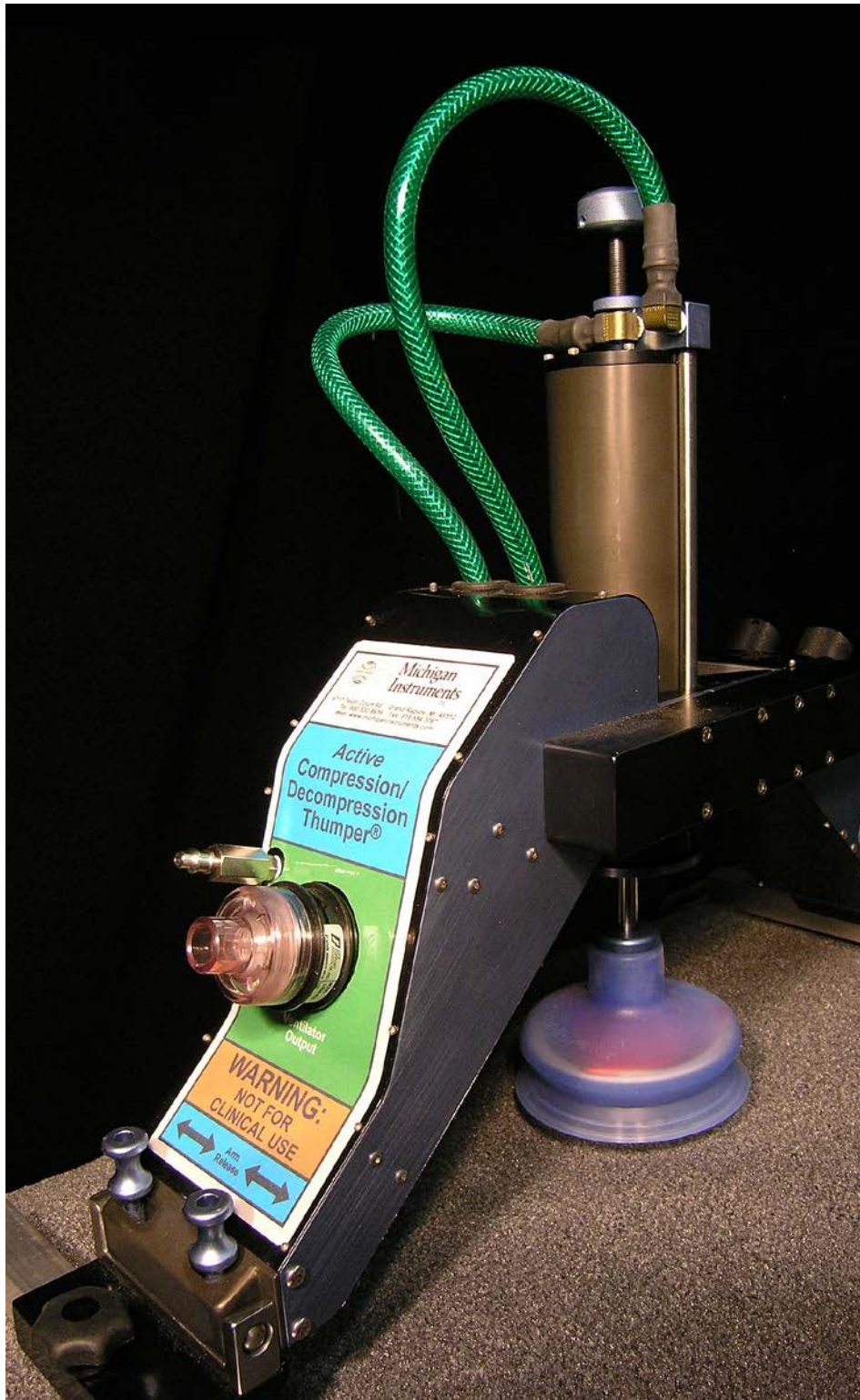
Figure 9-13. Gas intake and outlet on the Suspended Animation ACDC Thumper.
