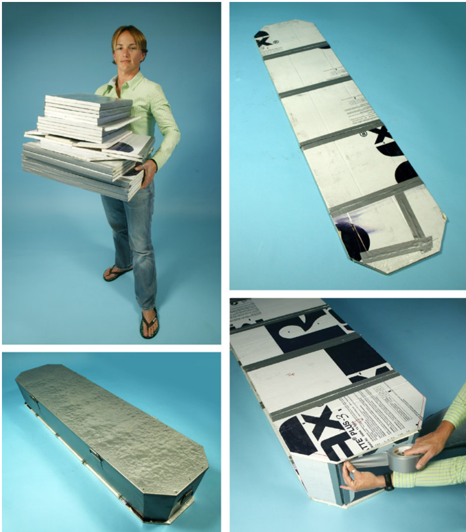
Figure 17-2. Unfolding and taping pre-cut foam board around a Ziegler box.
