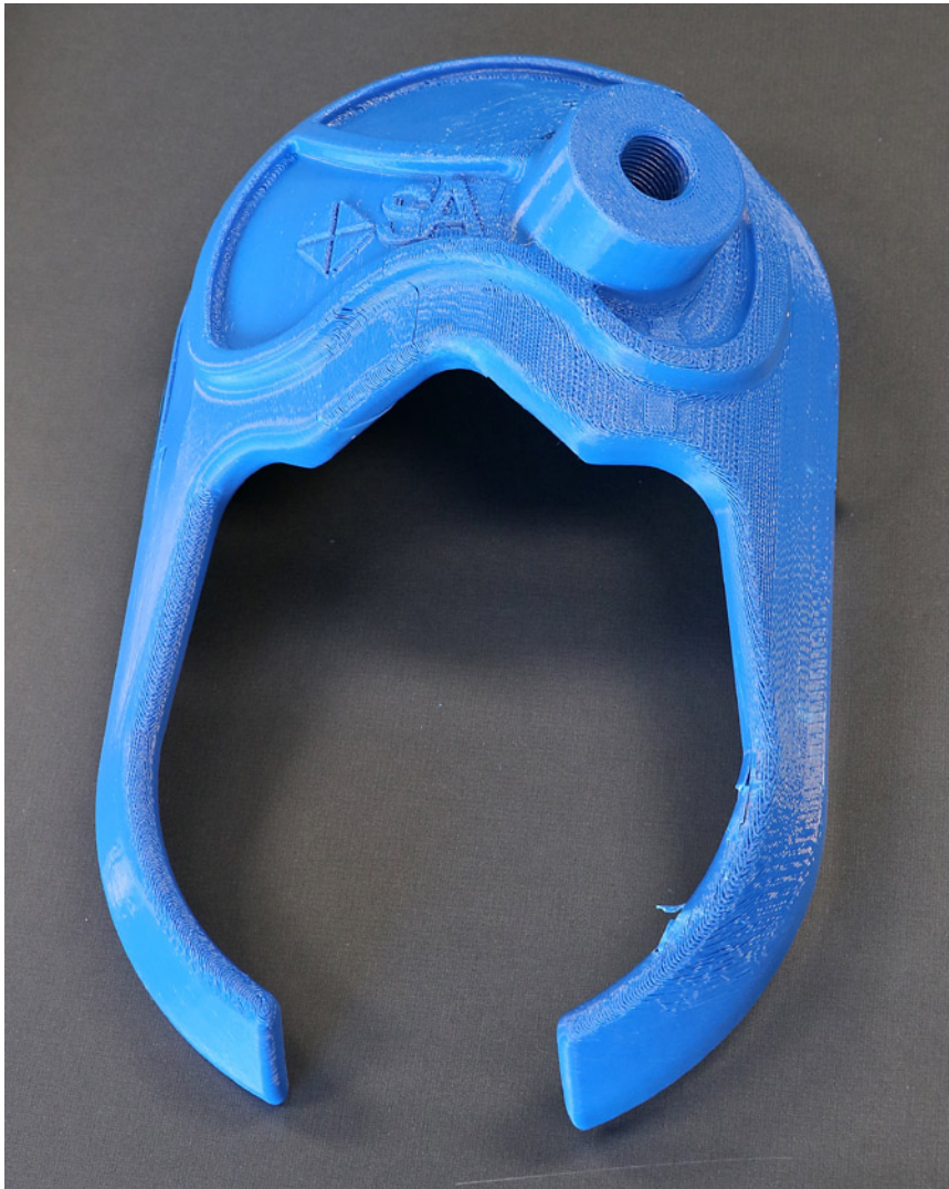
Figure 11-5. A mask to promote cooling of the head. Water is introduced in the threaded bushing and is released via perforations underneath the mask.
