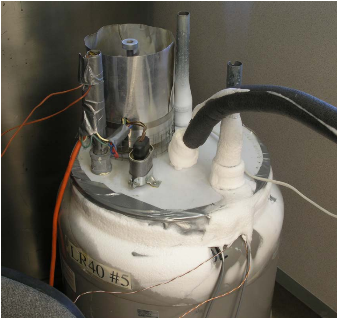
Figure 19-2. A neuro cooldown dewar at Alcor. Frost has accumulated from water vapor in the air while cooldown is in progress.
