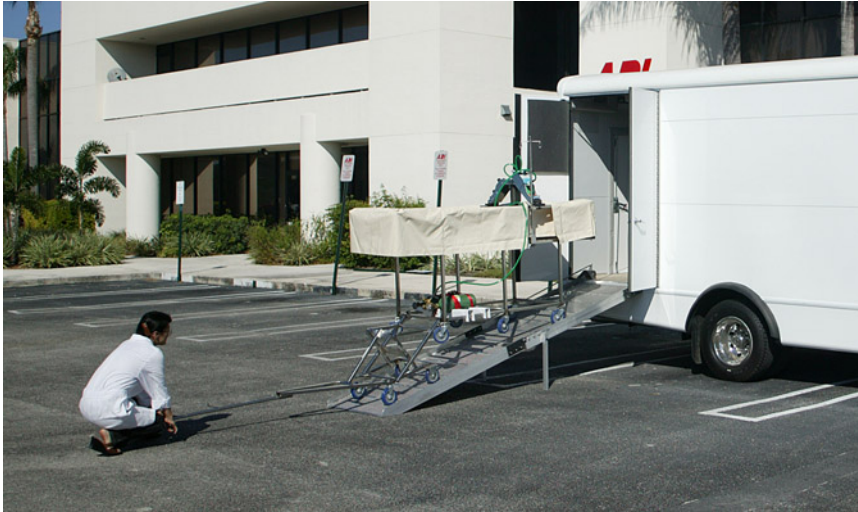
Figure 17-17. With a remote-controlled winch and a levelling linkage, the Suspended Animation vehicle could be loaded by one person through its side door, but the arrangement was not popular.
