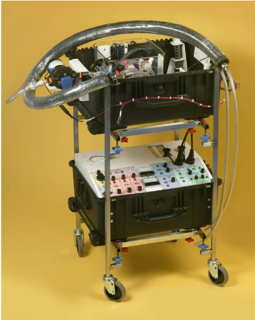
Figure 12-5. The LV2 liquid ventilation assembly designed and fabricated at Suspended Animation and demonstrated in 2007. The control panel in the lower Pelican container could be lifted out so that ancillary items (such as the infusion pump and insulated delivery tube) could be stowed below it for transportation. Lids of the Pelican containers were removable, and the stainless-steel frame was disassembled for shipping in a separate box. The concept of a frame was discontinued in LV3 in favor of a simpler arrangement in which the two Pelican containers were stacked and a small wheeled subframe was added to the lower container. LV2 used a more powerful suction pump than LV1, but infusion was provided by the same small submersible pump as in LV1.
