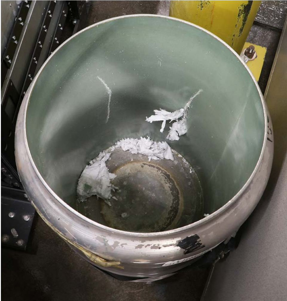
Figure 20-31. The interior of a small dewar after the interior shell has ruptured.
