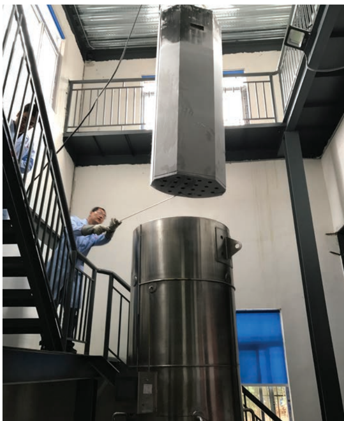
Cooled-down patient in a metal container being lowered into a dewar for long-term storage in liquid nitrogen
