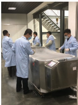
Patient in cool-down box being cooled to liquid nitrogen temperature prior to being placed in a dewar for long-term storage
