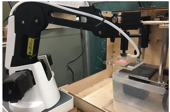
Robotic arm stacking layers of 2D tissues. (Photo courtesy of Gideon Ukpai, UC Berkeley)
