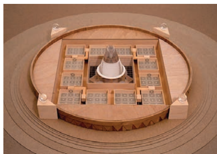
Model of Timeship viewing the lower cryostorage area divided into twelve communities. The hierarchy of Neighborhoods and Communities allows for security and redundancy. The inner square is for LN 2 storage and cryogenic equipment.
