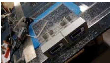
Refractometers after Mounting (Whole-Body System)
