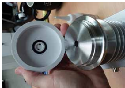
3D-Printed Adapter (left) for Neuro Refractometer
