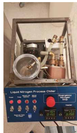
Liquid Nitrogen Process Chiller
