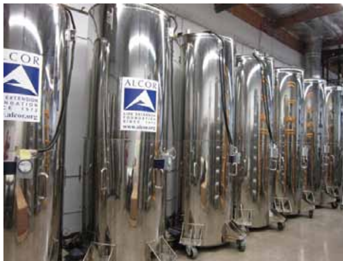
Bigfoot dewars at Alcor, September 2014. All but leftmost are the newer, taller type. Photo Credit: R. Michael Perry, personal collection
