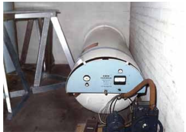
Steven Mandell’s capsule at CSNY’s facility in Coram, NY, the last and most advanced capsule manufactured by Cryo-Care. The closed end is forward and is where liquid nitrogen was introduced and vacuum pulled when necessary. A vacuum pump is hooked up (brown hose).
