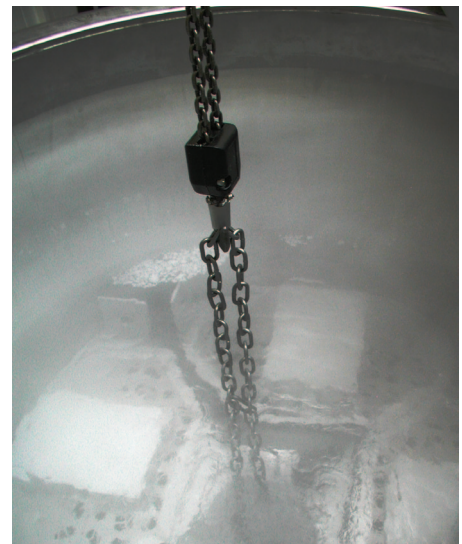
Water vapor creates a mist partially obscuring the arrangement of four wholebody pods and a central neuro pod in a bigfoot Dewar. The pods are perforated to allow liquid nitrogen to enter them when they are lowered into the Dewar. A chain hoist is used to lift and lower each pod.
