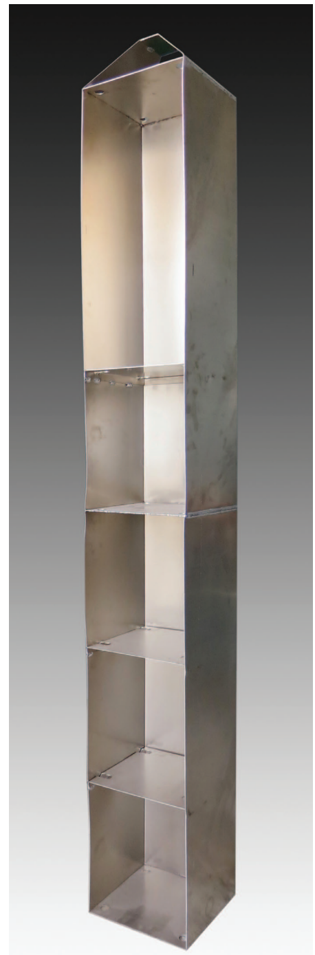
The "neuro column" is intended to store five cephalons in neuro cans, each of which will be wired into place on its shelf. Theoretically the column could store six cans, but the top section is usually left empty as a safety precaution in case of unexpected liquid nitrogen boiloff.
