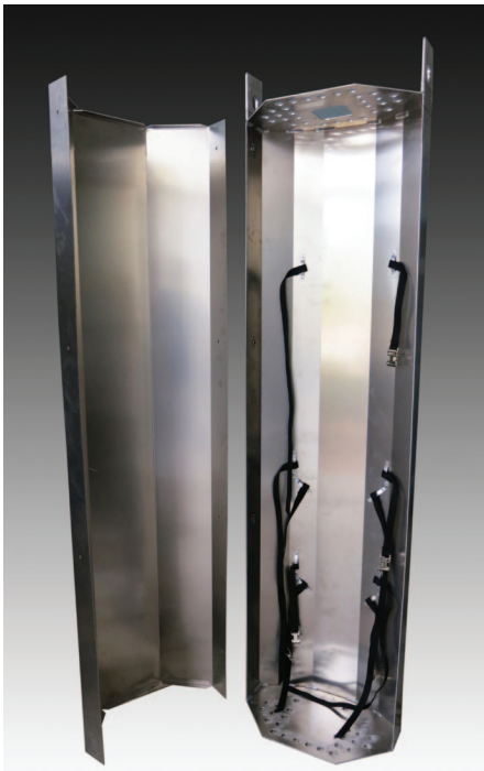
A “pod” is an aluminum clamshell to contain and protect a human patient while immersed in liquid nitrogen. The two sections of the pod are held together with sheet-metal screws. The “ears” at the top are to lift the pod before it is lowered into a Dewar. The two sections of a pod are shown here separated. Straps in the right-hand section will hold the patient in place.
