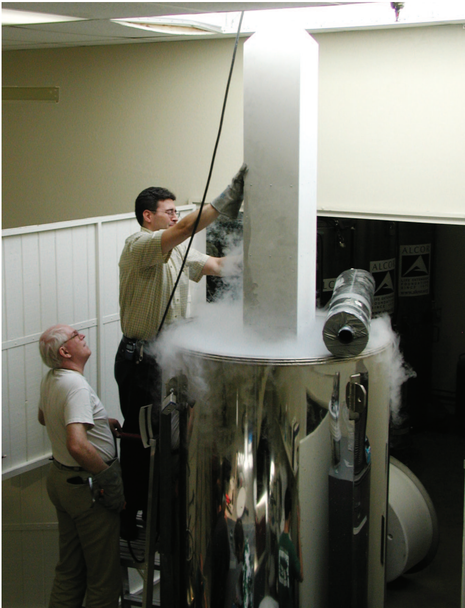
The central box-shaped aluminum pod can contain six neuropatients, each in its separate cylindrical container, stacked vertically. This sequence shows the center pod being lowered into a dewar after a neuropatient has been added.
