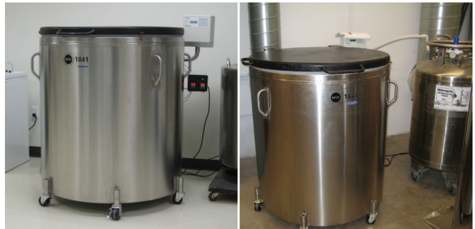
Fig. 13. (Left) ITS Neurodewar with dual redundant temperature controllers and displays on the right side of the unit. (Right) Neurodewar in operation at Alcor, maintaining an internal temperature of -140°C. The unit automatically refills itself from the connected liquid nitrogen tank.
