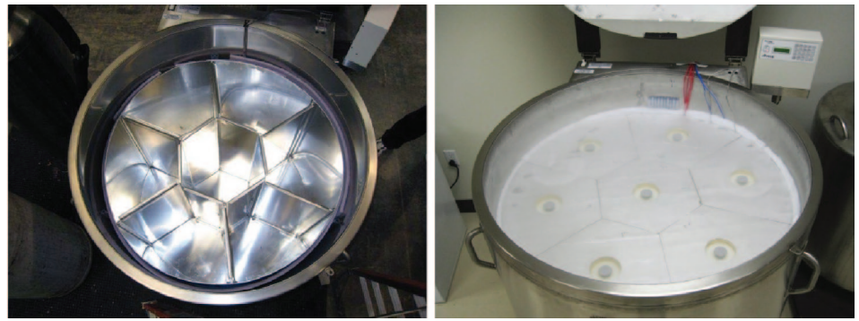
Fig. 12. (Left) ITS Neurodewar under construction, showing storage chamber with seven storage compartments. (Right) Neurodewar in operation with main lid open, showing closed storage compartment lids.
