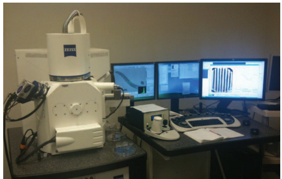
Scanning electron microscope which can automatically image a complete wafer of ultrathin sections producing volume images with resolutions of 5x5x30 nanometers – sufficient to trace the finest neuronal processes and synaptic connections.
