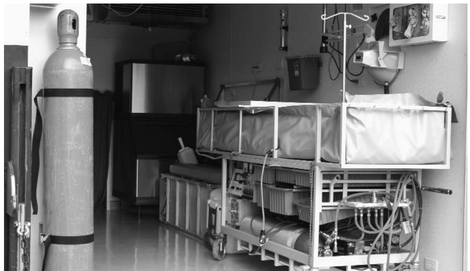
Inside of transport vehicle, showing MRC, oxygen tank, and ice machine in far right corner
