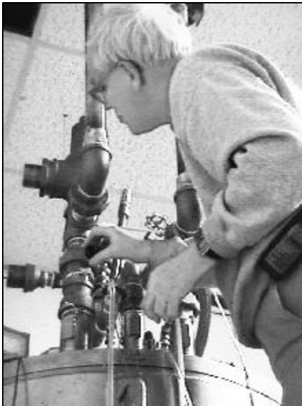
Hugh Hixon adjusts fittings on top of the pressure vessel of the new system.
