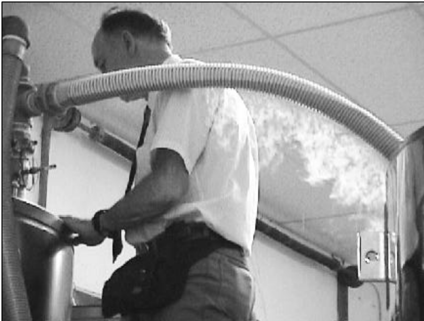
After that things get more routine—but there's still a lot of work to do. These pictures were made Dec. 15. The suction pump is being used to transfer liquid nitrogen from the bigfoot 8 dewar into the pressure vessel, watched by Alcor CEO Fred Chamberlain. Afterward, bigfoot 8 is refilled with liquid nitrogen, its thick foam lid resting on top.
