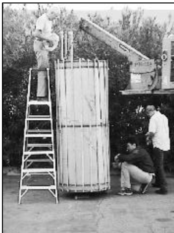
Wooden slats are fastened around it to protect against contact with the container it’s going into.
