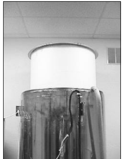
After that things get more routine—but there's still a lot of work to do. These pictures were made Dec. 15. The suction pump is being used to transfer liquid nitrogen from the bigfoot 8 dewar into the pressure vessel, watched by Alcor CEO Fred Chamberlain. Afterward, bigfoot 8 is refilled with liquid nitrogen, its thick foam lid resting on top.
