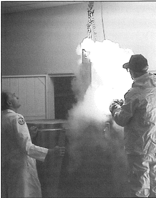
“A”’s Transfer to a Bigfoot Dewar After Slow Cooldown to Liquid Nitrogen Temperatures
