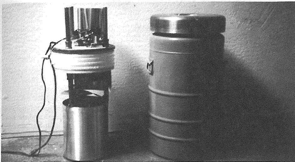
The neuropatient cooldown apparatus, here next to its container. . .
