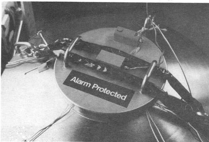
Photo (Above) shows the alarm switch boxes on the top of the dewar lid. The chain and lock are for security.
