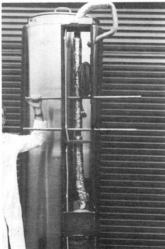
Photo B (right) illustrates the use of short pipe sections to facilitate lowering and raising the pump assembly in the dewar.
